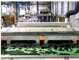
Photo 7: A multi-stage production process is the surface treatment by so-called electropolishing, among other things in basins with an acid mixture (photo). Here, the roughness of stainless steel surfaces is reduced, resulting in extremely smooth surfaces. This is important for baskets and inserts used in medical and laboratory technology. (Photo: Miele)
