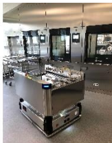
Photo 1: Heart and soul of Steelco's automatic transfer system: a transport robot which autonomously loads and unloads machines. (Photo: Steelco)
