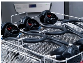
Photo 2: There is space for two baskets in the special-purpose washer, for example for 6 air regulators (above). On the lower level, breathing masks can also be washed and dried. (Photo: Miele)
