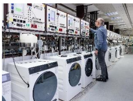
Photo 2: Endurance test in the laboratory: Miele tests appliance models for a service life of up to 20 years. (Photo: Miele)
