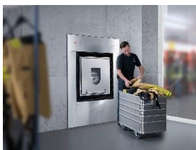
Photo 1: Washing machines with two doors reprocess firefighting protective suits. The two separated sides prevent any redeposition of soil on cleaned textiles. (Photo: Miele)
