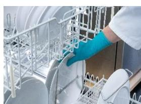
**Photo 3:** Diana Klapper attaches "contaminated" stainless steel test pieces to plates using special holders. The microbiological result is determined in five separate washing tests that are then used to calculate an average value. (Photo: Miele)
