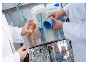
**Photo 2:** Is everything dry? Once the programme is complete, every single reusable cup is put to the test. Damp reusable cups are a hygiene risk and can transmit germs. (Photo: Miele)
