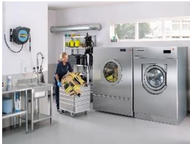
Photo 1: Miele Professional laundry machines can be used to reprocess a fire brigade's entire range of protective equipment, such as multiple-layer trousers, jackets and helmets. (Photo: Miele)
