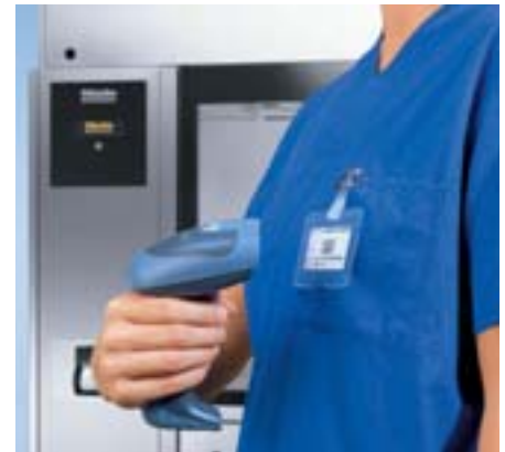
Scanning in of personal barcode after load release
