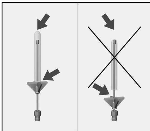
If the tip of an injector nozzle touches the bottom of a piece of glassware, the plastic support has to be pushed upwards.
